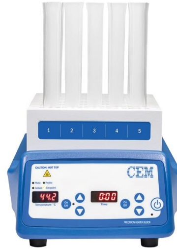
Condition samples in heater block
